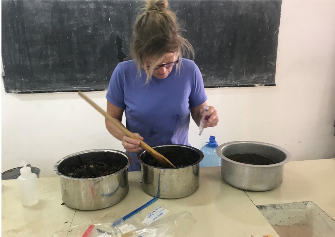
Figure 6. The samples were rinsed three times and a visual scan for microplastic particles was done before sieving the samples through three sieves with different sizes.
