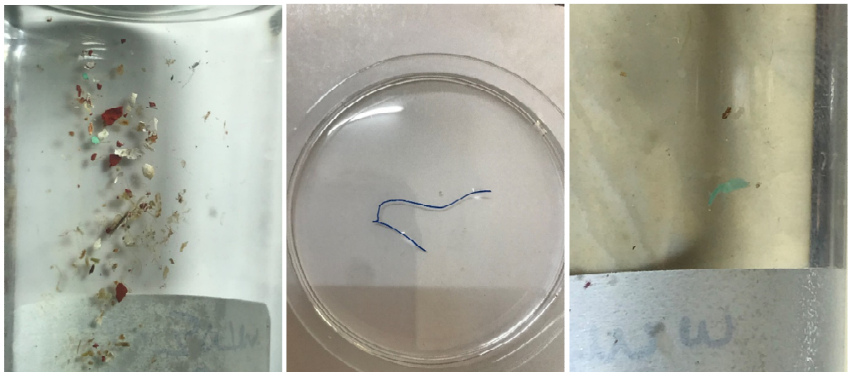
Figure 10. Pictures of different types of microplastics found in the samples, from left to right several fragments, a thread and a film.
